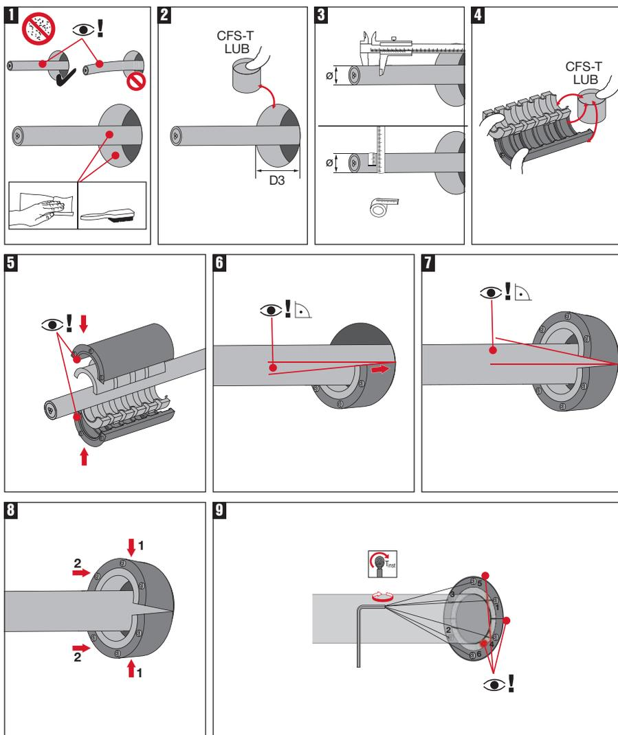
1. Make sure the cable is supported for a straight penetration. Clean the cable and the opening area (i.e. for dust).
