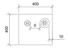
\*) Valid also for flexible and rigid plastic conduits (Polyolefin, PVC),  $\emptyset$  < 32 mm and for bundle of plastic conduits,  $\emptyset$  < 100
